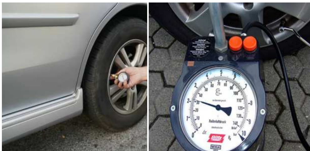
Figure 3.7: Measuring vehicle tyre pressure
