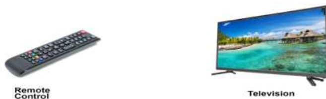
Figure 2.36 Example of simplex transmission
