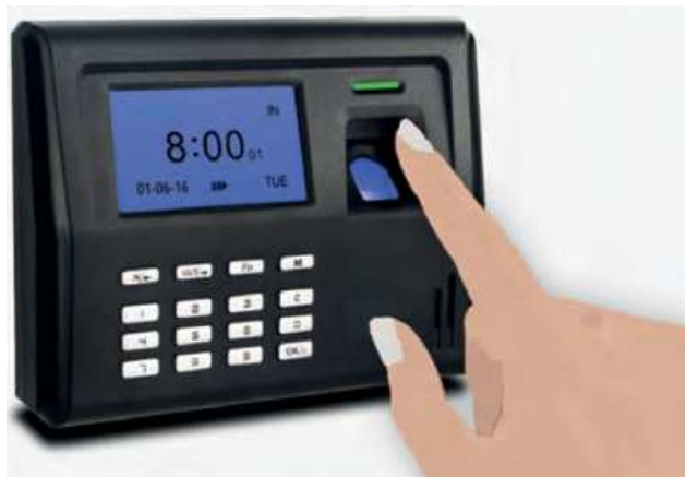
Figure 1.18: Digital Identity Attendance controlling device using fingerprint
