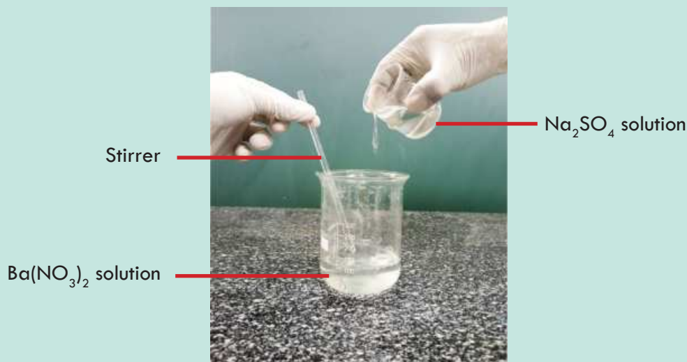
Figure 1.6 Double displacement reaction between \text{Na}_2\text{SO}_4 and \text{Ba}(\text{NO}_3)_2
