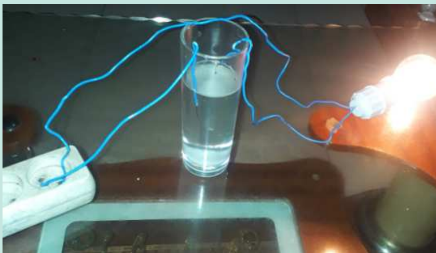
Figure 4.6 Setup for electrolytic conductivity test.
