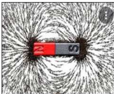
Figure 7.17 Plotting magnetic field lines using iron filings
