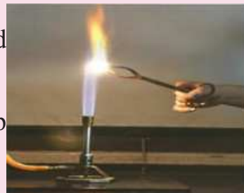
Figure 3.4 Burning of magnesium in air
